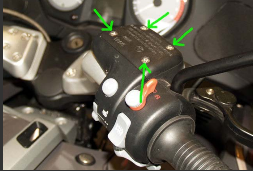
The front master cylinder on the RT has 4 screws.
